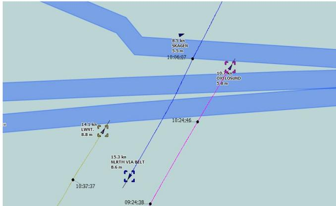
Figure 2. Display of a subset of registered AIS messages: position, time stamp and speed over ground for a vessel operating in and around the pipeline surveillance zone.
